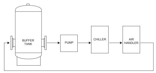
OTHER VALVES AND ACCESSORIES REQUIRED FOR SYSTEM INSTALLATION ARE NOT SHOWN.
